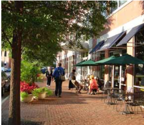
Expanding brick areas to include the whole sidewalk helps provide definition to places where outdoor dining or other special use of the sidewalk is encouraged.
